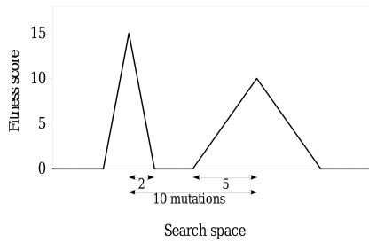
Figure 1: Two-peak fitness landscape , with one narrow peak of high fitness (Peak 0), and one broader peak of lower fitness (Peak 1). The fitness score is relative, and the width and distance between the peaks are given in terms of Hamming distance. Diagram adapted from Wilke (2005).
